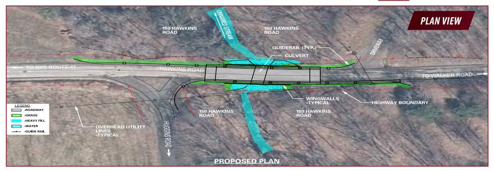
The Town of Sanford, in cooperation with the New York State Department of Transportation (NYSDOT), is in the process of developing preliminary plans for the replacement of the culvert carrying Hawkins Road over an unnamed stream immediately east of Huggins Road.
